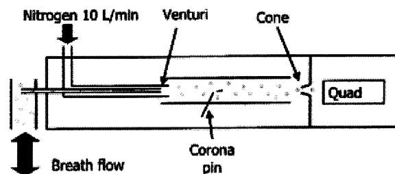
Fig. 11. Schematic diagram of the APCI source. Reprinted with permission from Ref. [135].
